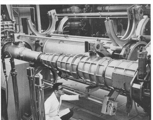
REVOLVING TEST SECTIONS are a unique design feature of the new hypersonic wind tunnel. The Mach 7.5
